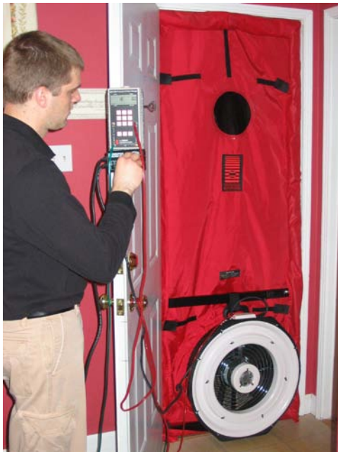
Using a blower door to assess energy efficiency in a residential building
