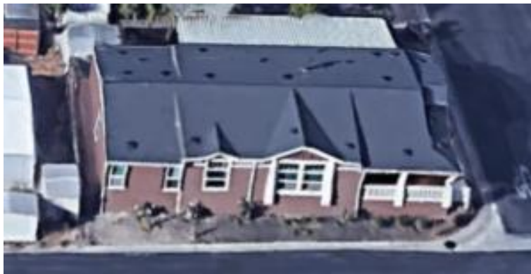
Figure 13: Example of a newer residence. Despite south-facing aspect and no shade, numerous different rooflines from dormers and other structural elements, as well as numerous vents, significantly limits the space available for rooftop solar
