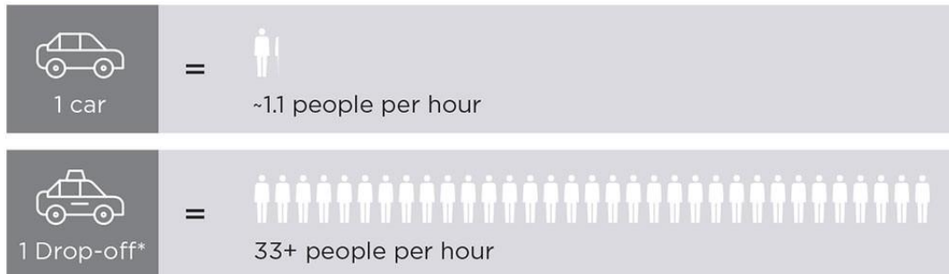
The chart above illustrates how on-street parking allows around 1.1 person to access the curb per hour, while pick up and drop off zones allow over 33 people to access the curb per hour. Graphics by Haisam Hussein; graphs courtesy Stantec's Urban Places, based on NACTO data.
